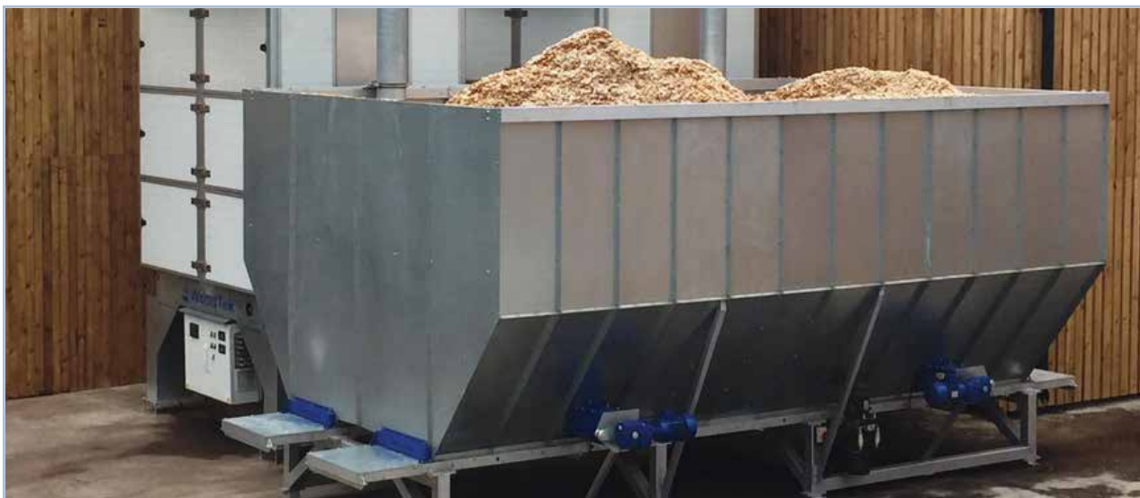
2 x Eco T4 dryers with a 55m 3 fuel store hopper
