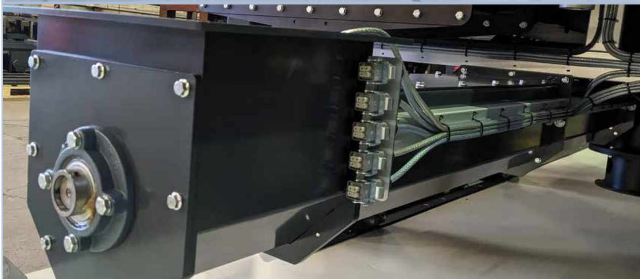
Where possible electrical installation is completed before delivery to site which saves installation time and cost. Power and signal cables can be plugged together during installation proving a Plug and Play solution
