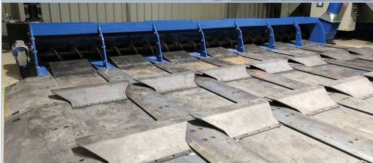
Walking floor fuel store Installed in Yorkshire to provide feedstock to a single Eco T2 Plus dryer
