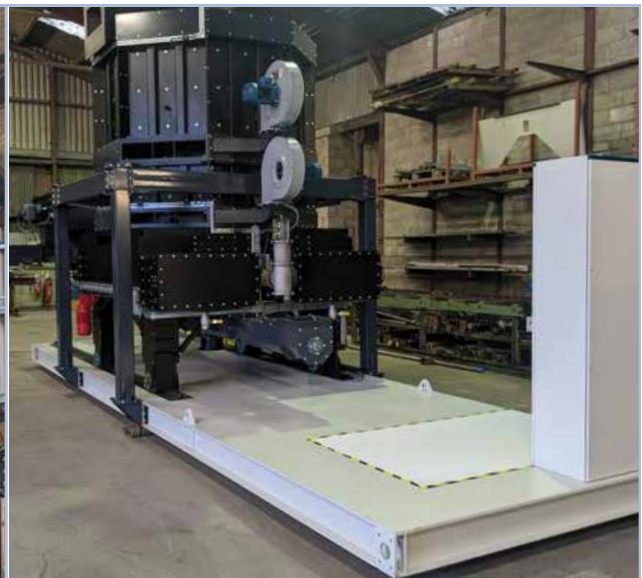
C1000 rear view showing fuel in-feed and control
