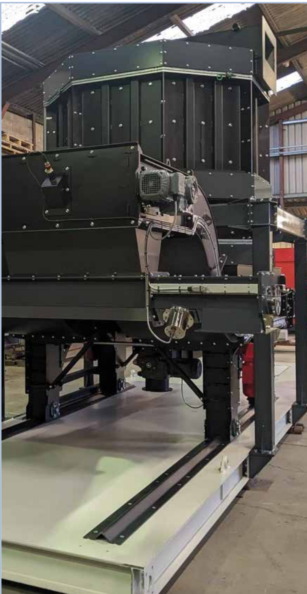
C1000 - Front view with biochar metering auger
